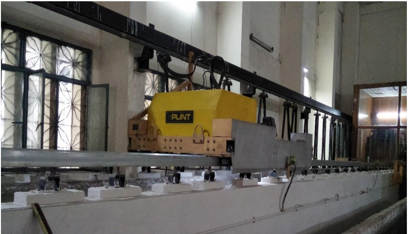
Figure 2: View of the Trolley on rail track of calibration channel and the control room
