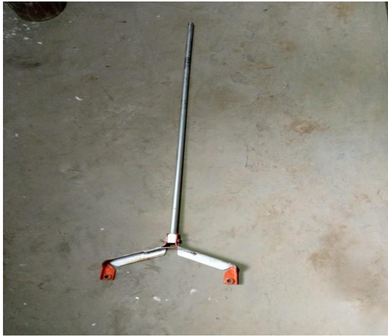
Figure 4: Specially manufactured hanging rod for coupling of ADCP with Trolley
