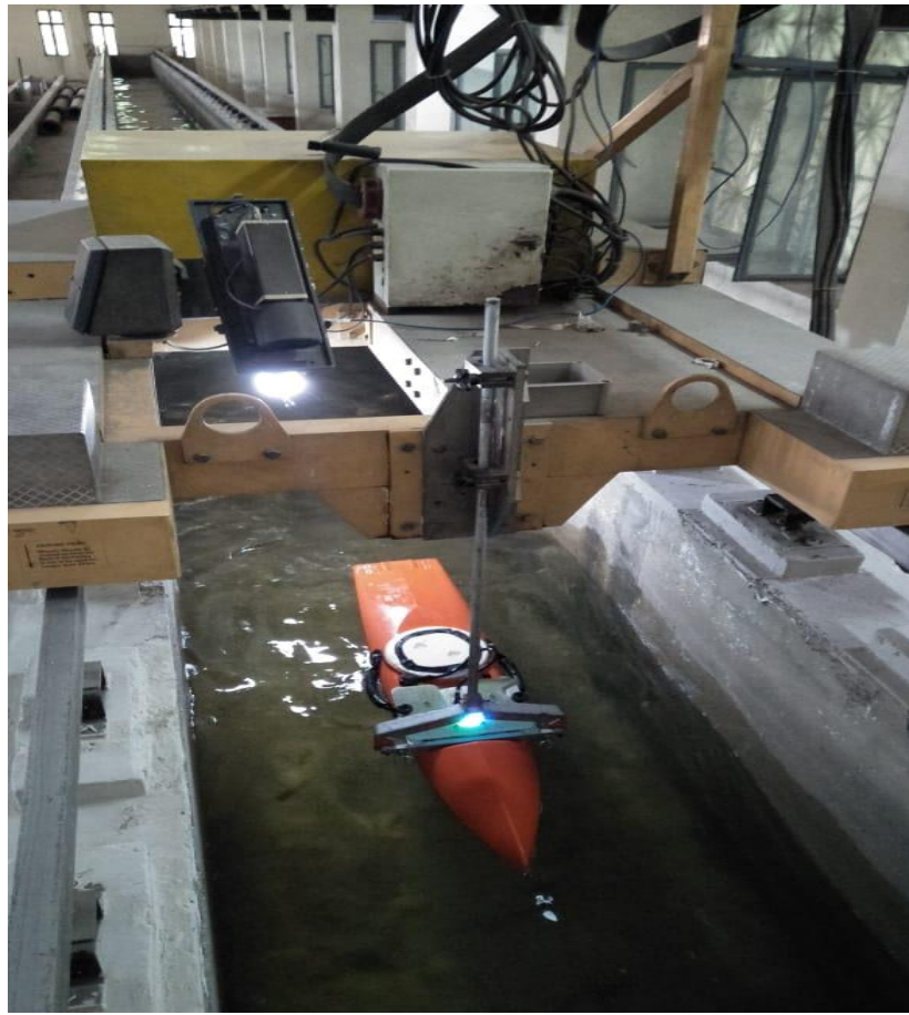
Figure 6: View of ADCP boat coupled with trolley
