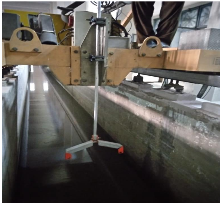
Figure 5: ADCP coupling rod attached with Trolley
