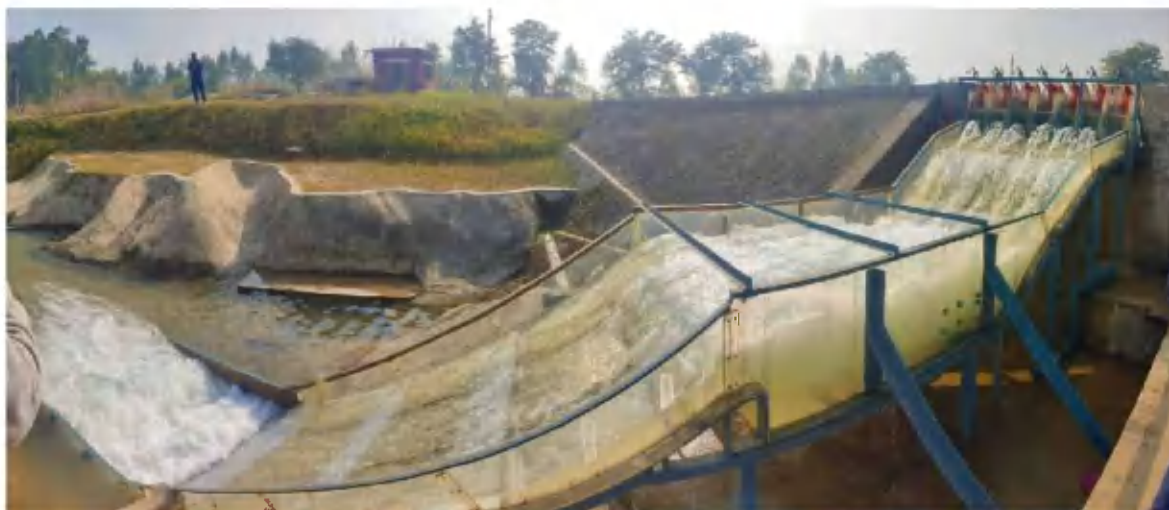
Scale Down Physical Model of Mohmand Dam Spillway
