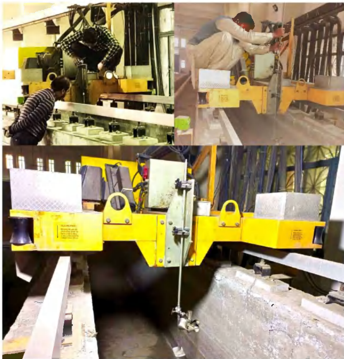
Glimpses of Testing and Calibrating the AA Type Current Meters Using Tow Trolley
