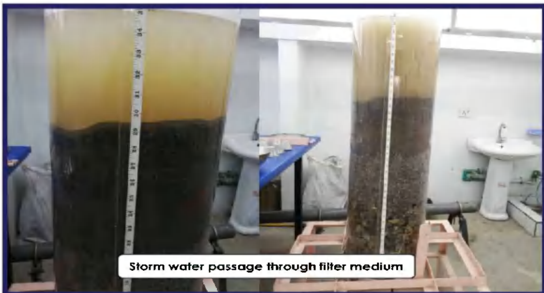
Lab Experiment to Select best filter medium for Storm water
