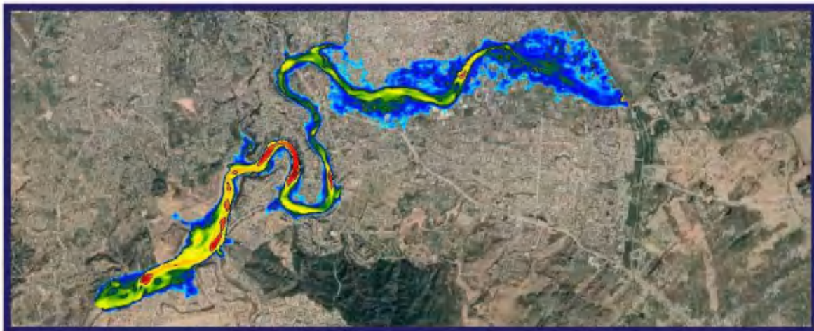
Two Dimentional Unsteady Flow Simulation with overlay on Base Map
